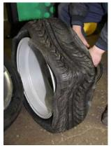
Note: Tires should never be subjected to a vacuum to eliminate the oxygen. Distorting the tire as shown in the accompanying picture can be as detrimental to the internal structure of the tire as running over potholes and road hazards.
